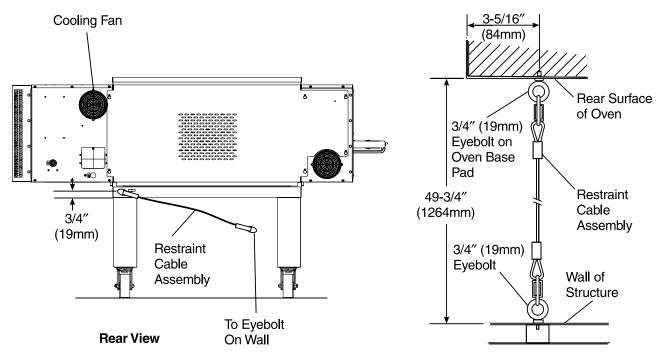
Figure 2-8. Restraint Cable Assembly Installation
